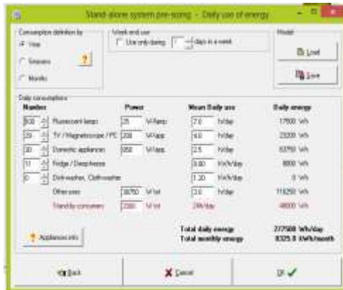
Fig 4: Energy Needs Computed In PVsyst.
