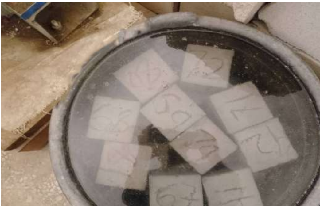
Figure 4. Curing of cubes
