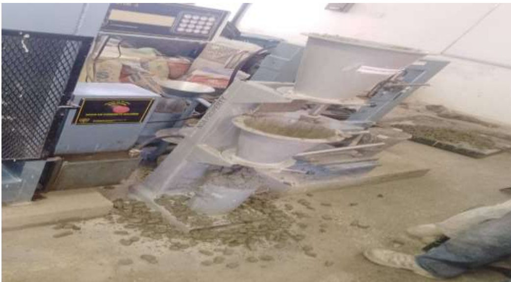
Figure 2. Compacting factor test
