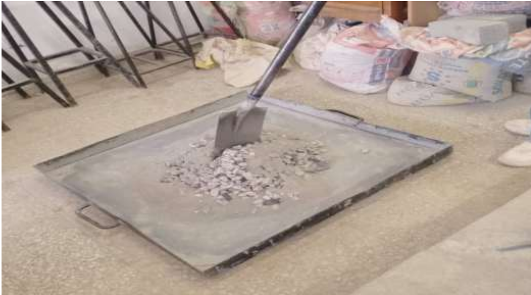
Figure 1. Mixture of cement + ceramic waste, fine aggregate, and coarse aggregate + shredded tyre
