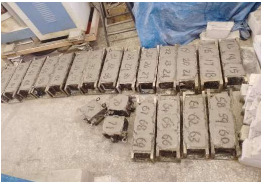
Figure 3. Concrete cubes before demoulding
