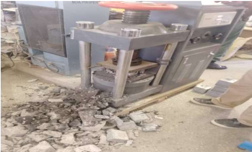
Figure 5. Crushing of cubes
